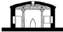
Fig. 9: Above ground unicameral garadams
