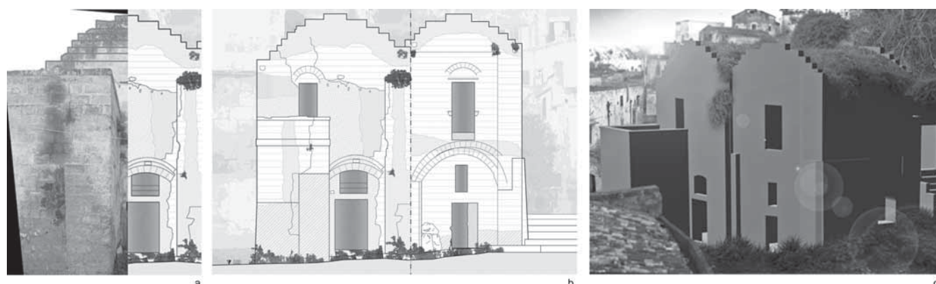
Fig. 5. To find necessary to integrate and interpret data: frames, designs, analysis of degradation, processing 3D
