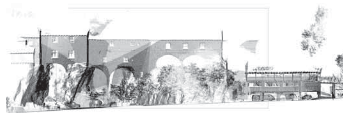
Fig. 12 . laser scanner survey – vertical section of the generated point cloud.
