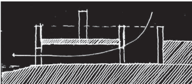
Fig. 3. cave section – ventilation scheme. (Drawing: HC)
