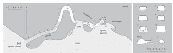
Fig. 3.06) Ani, plan and transversal section of the Orchard tunnel (or Secret Gates) (topography R. Bixio, V. Caloi, V. Castellani, M. Traverso; drawing R. Bixio).
