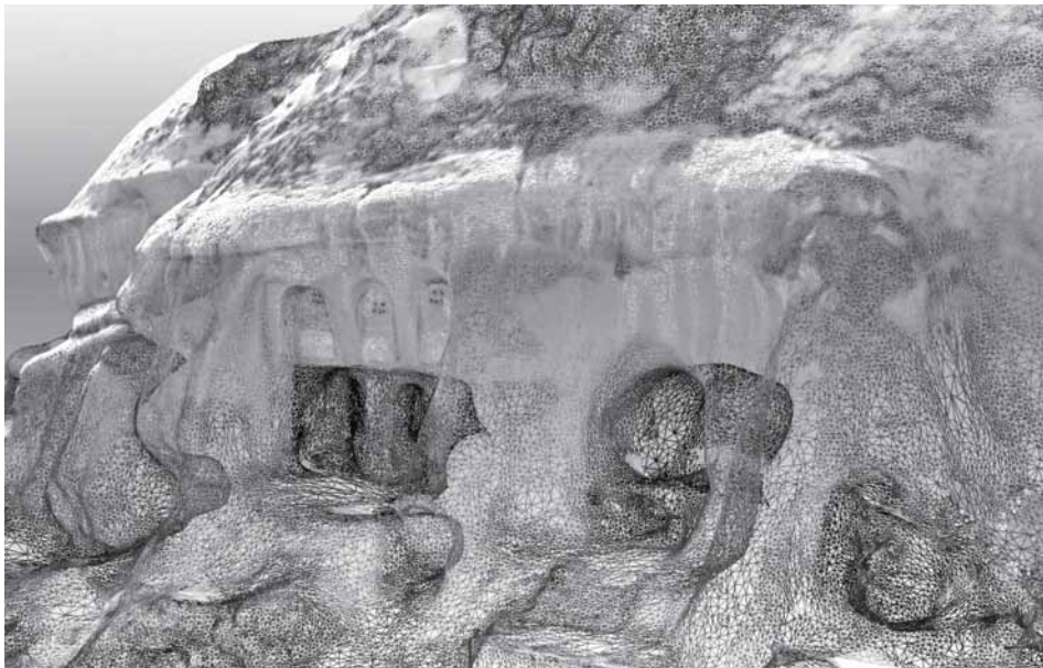
Fig. 1 Durmus Kadir Kilise, Mesh of the reconstructed image. The texture was removed to better understand the geometrical structure of the object.
