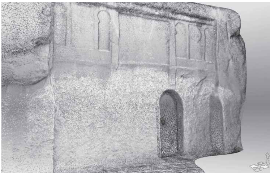
Fig. 2 Church of St Jean in Gulşehir, Mesh of the reconstructed image. The texture was removed to better understand the geometrical structure of the object.
