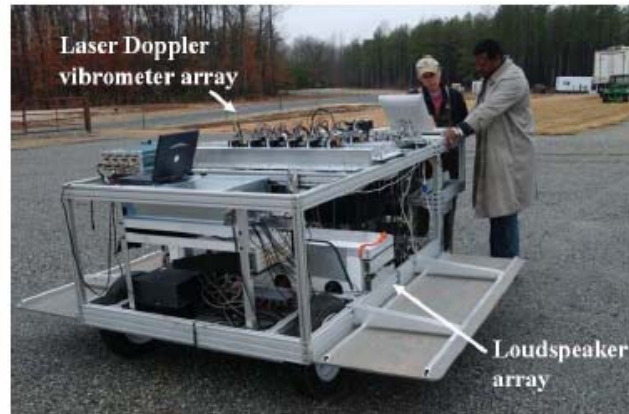
Figure 12 Photograph of the moving platform with multiple Laser Doppler Vibrometers [R12].
