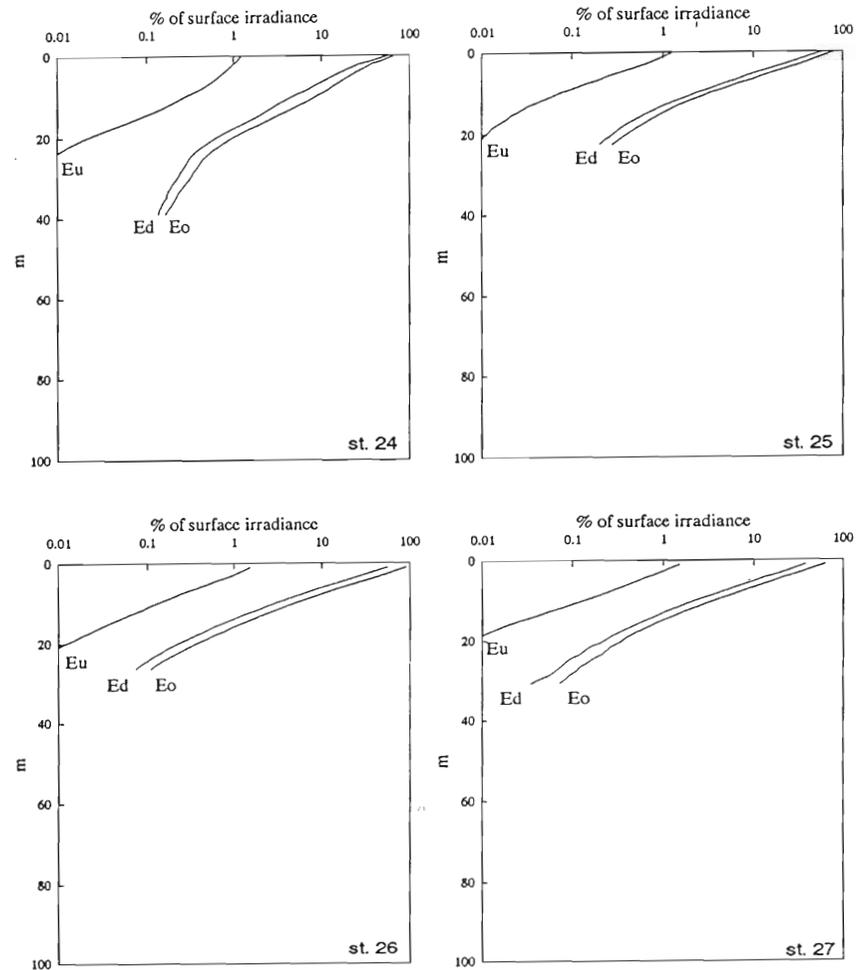
Fig. 28 - Underwater scalar ( $E_o$ ), downwelling ( $E_d$ ) and upwelling ( $E_u$ ) quantum PAR irradiance normalized to surface downwelling irradiance.
