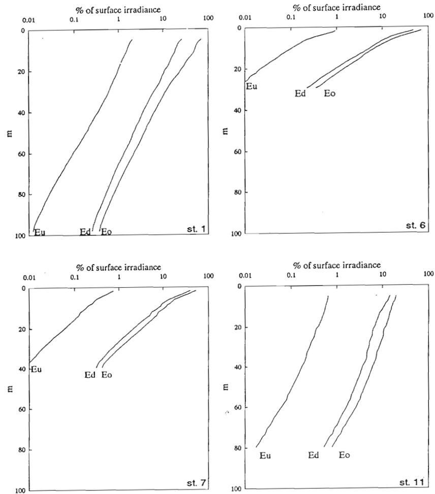
Fig. 26 - Underwater scalar (Eo), downwelling (Ed) and upwelling (Eu) quantum PAR irradiance normalized to surface downwelling irradiance.
