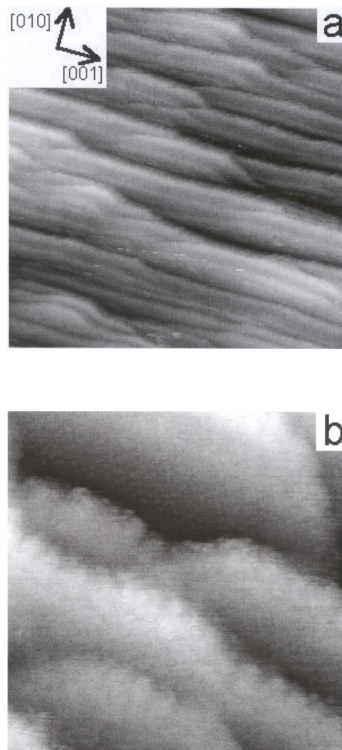
Fig. 4. STM images collected after an exposure of 150 s (a) and 300 s (b) at p\text{O}_2 of 2 \times 10^{-7} , T 770 K. (a) 97 \text{ nm} \times 101 \text{ nm} , tunneling current 0.2, sample bias -0.3 \text{ V} ; (b) 27.7 \text{ nm} \times 26.9 \text{ nm} \times 1.7 \text{ nm} , tunneling current 0.2 nA, sample bias -0.3 \text{ V} .
