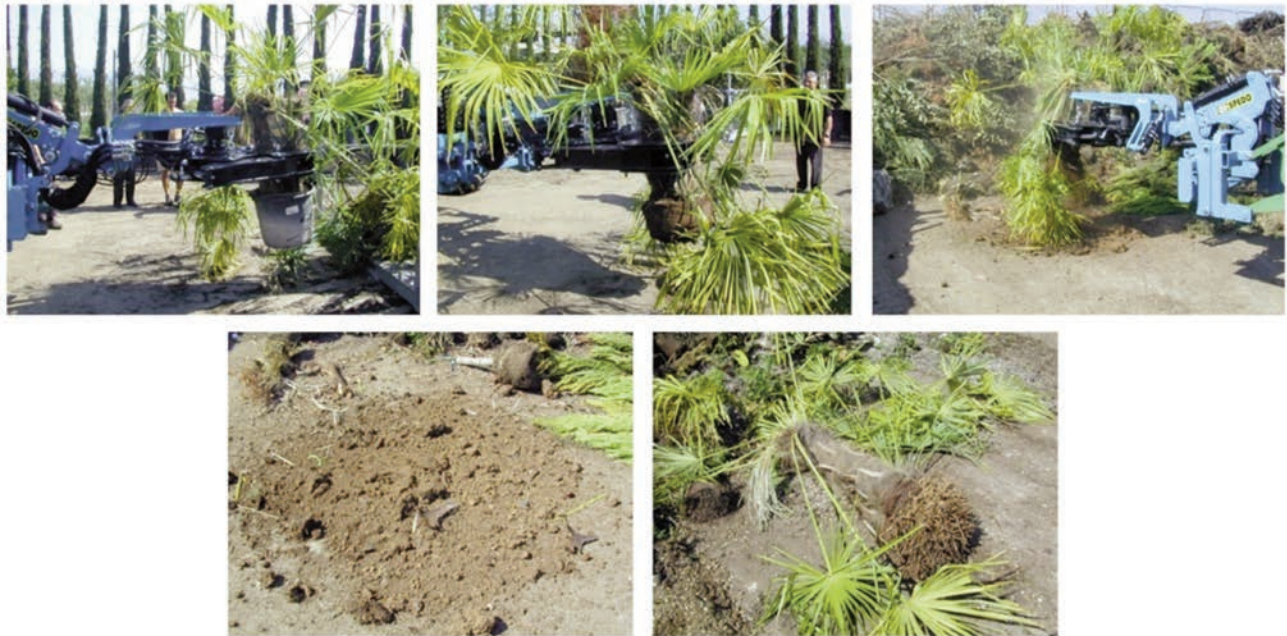
Figure 5. The operative logistics: grip the tree, containers recovery, shaking, heaping up the biomass.
