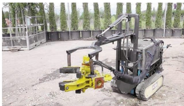
Figure 3. The “Unifi prototype” made of a small track-laying walking tractor equipped with a shaker clamp.
