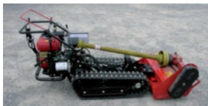
Figure 5. Fratelli Camisa - TP 480H Crawler tractor with guidance from the ground and power takeoff.
