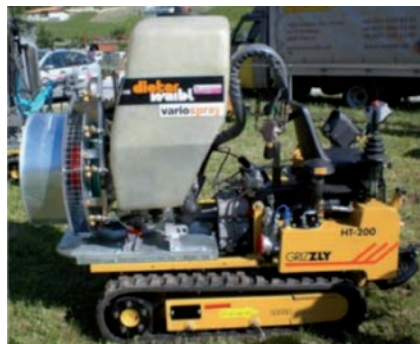
Figure 4. Ro.Da.G – Mini crawler tractor – HT 200 – The tank contains 25l, max flow rate 24l/m.
