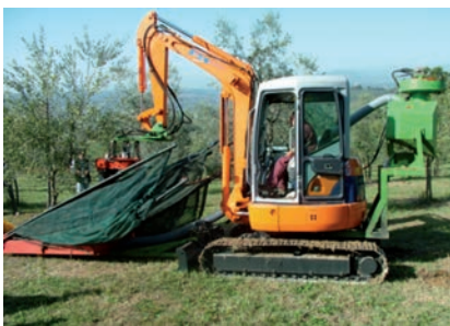
Figure 19. The integrated yard. The head shaker and the reverse umbrella on the front and the cleaner system on the back.
