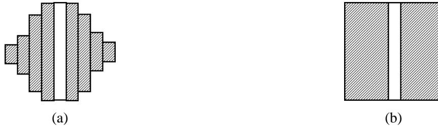
Fig. 3.37 - Different shapes of a vertical filtering window. (a) Negative exponential shape. (b) Classical square shape.
