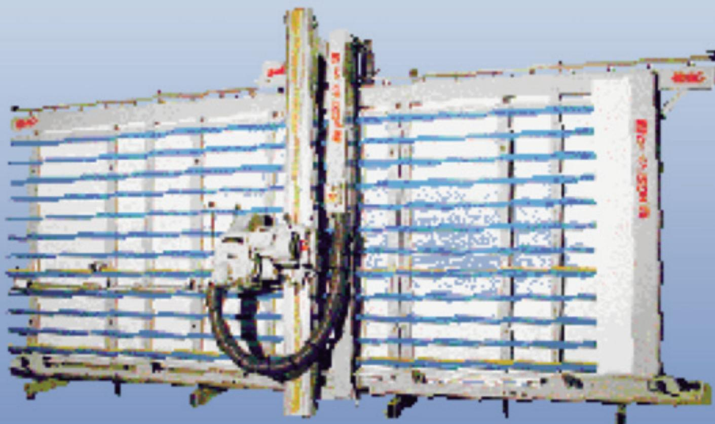
***New vertical panel saw/sizing machine
