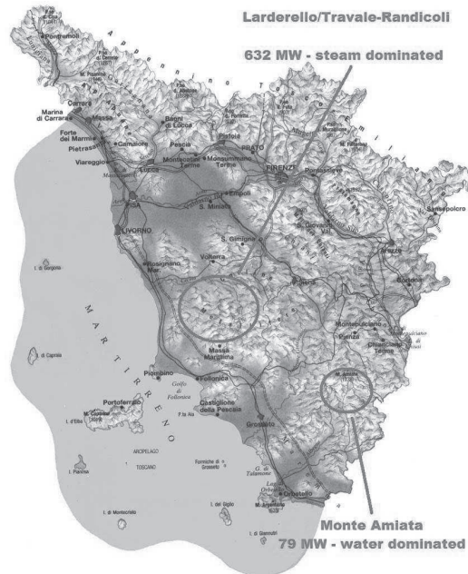
Figure 3: Location and size of geothermal power production sites in Tuscany, Italy
