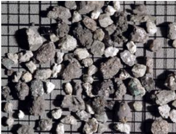
Fig. 30 Example of lunar regolith composed of fractured rock material ok parts with a size <1cm to 2-4 mm size. (photo by Randy Korotev, Mancuso et al. 2008)
