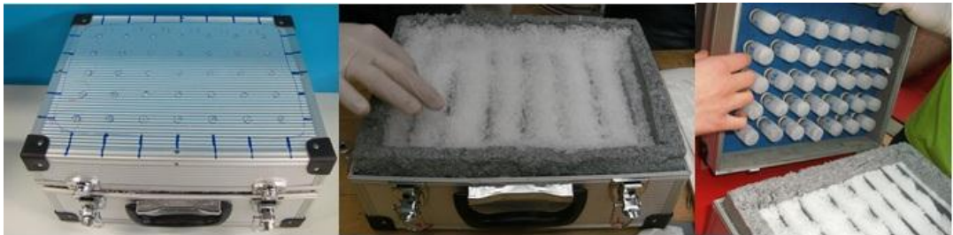
Fig.22 Three pictures of the Aluminium box and the collection tubes inserted in dry ice.
