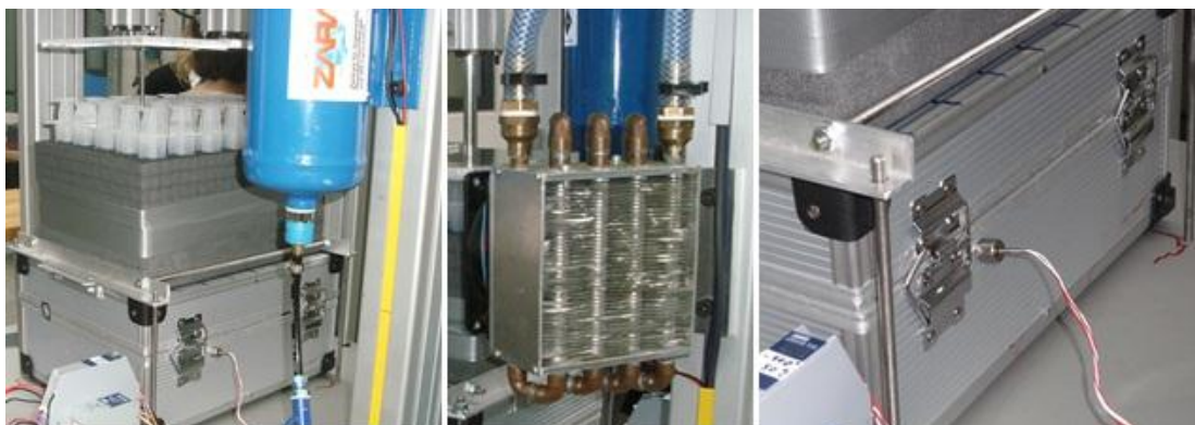
Fig.24 From left to right: overview of the set-up fixed on the capsule and of the metallic clamps, the thermostated serpentine and the probe to monitor the temperature inside the capsule.
