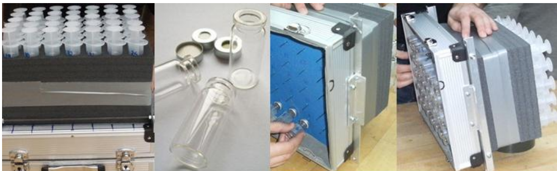
Fig.23 The 35 syringes and the polystyrene support on the top of the box. The needles reach directly the collections tubes.
