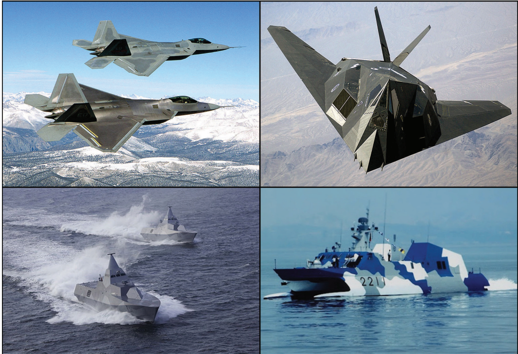
Figure 3.24. An example of “stealth” targets. The stealth technique is developed against \mu -wave radars and it is ineffective against HF radar systems.
