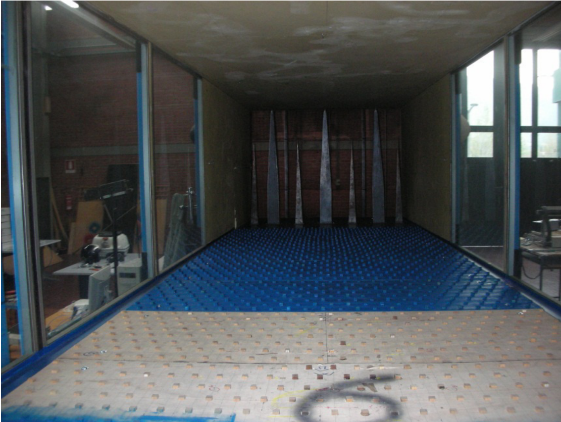
Figure 6.7 Atmospheric boundary layer facilities at CRIACIV
