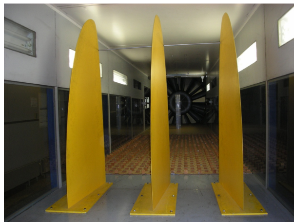
Figure 4.3 View of the model in the wind tunnel with turbulent facilities
