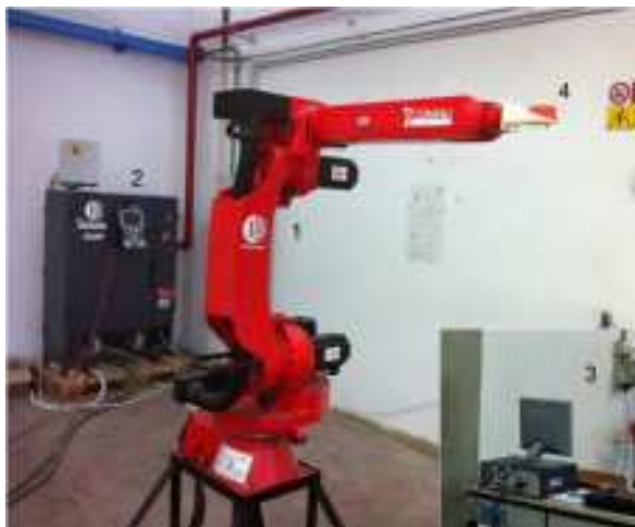
Figure 5.1: Hardware-In-The-Loop test rig: 1) industrial robot Comau SMART-SiX 6-1.4, 2) C4G control unit, 3) external Linux host, 4) IMU MTi-G by Xsens
