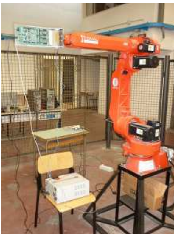
Figure 6.45: HIL test rig
