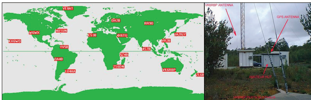
Figure 5.3. Map of HF beacon stations around the World and picture of the VK6RBP HF beacon located near Perth, Australia.
