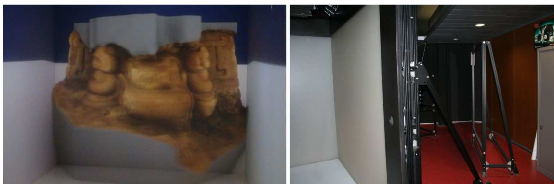
Fig. 19 – (left) Results of the developed simulation inside the CAVE. (right) Rear-projected displays used, with a mirror to reduce the room space requirements
