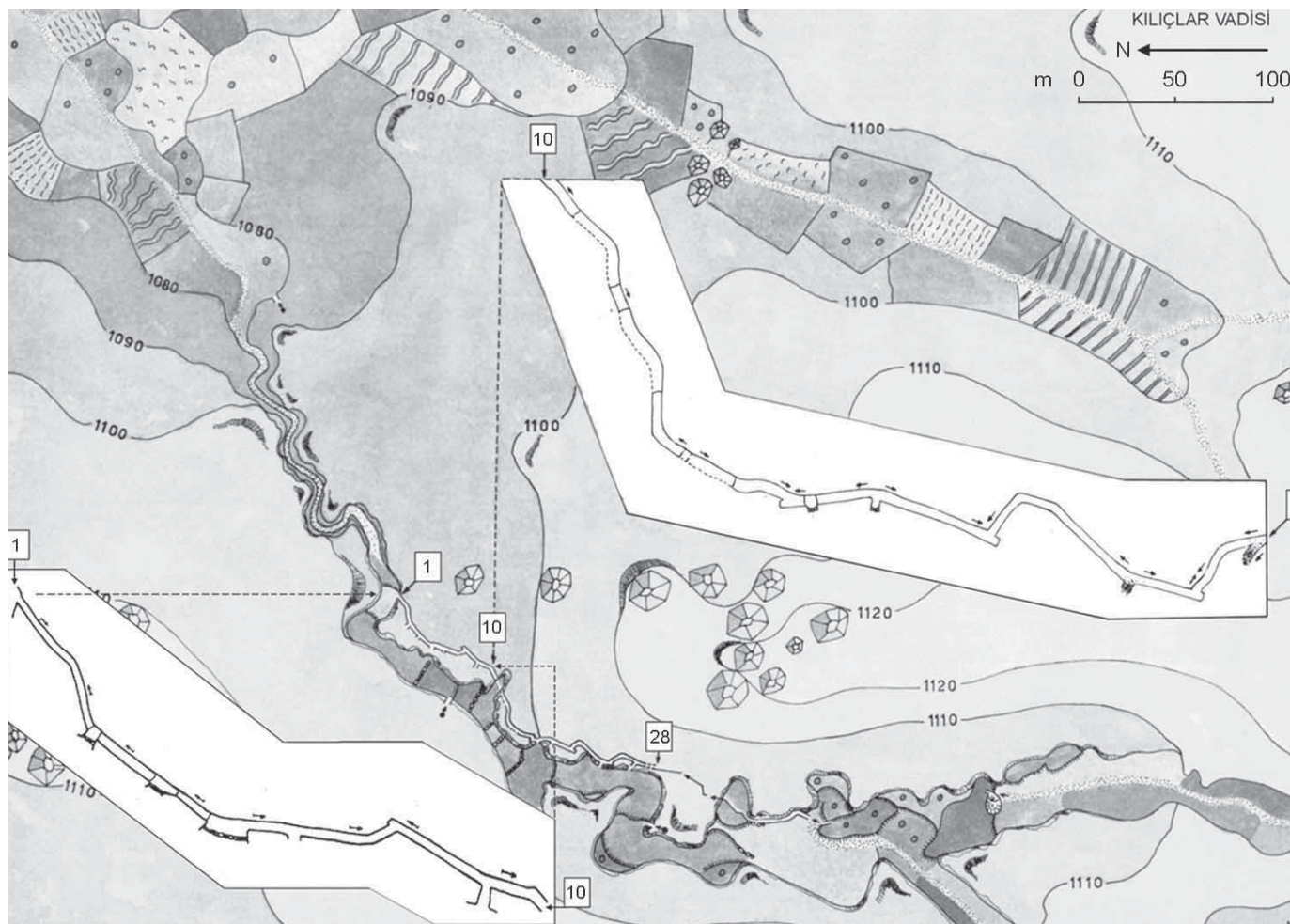
Fig. 20 Draining tunnels under the valley of Kılıçlar (drawing R. Bixio)
