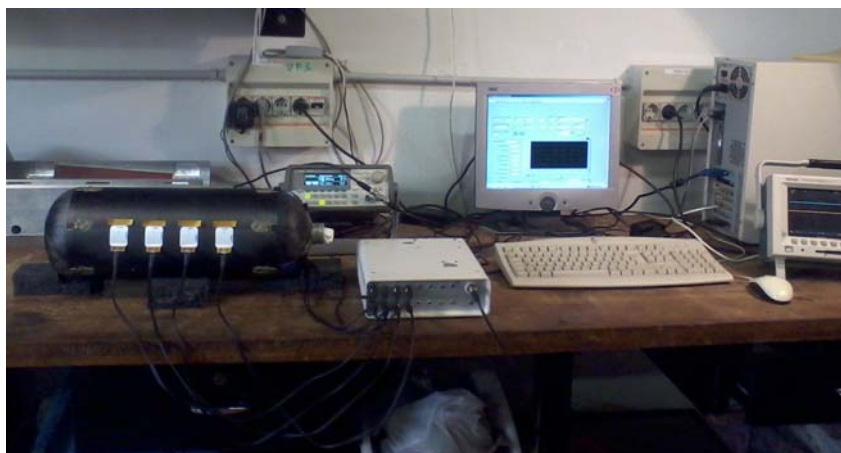
Figure 1 Programmable acquisition system for active SHM on COPV with piezopolymer interdigital transducers.
