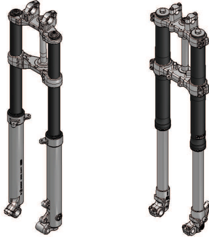
Figure 2.2: Comparison between a standard fork (left) and an up side-down fork (right).
