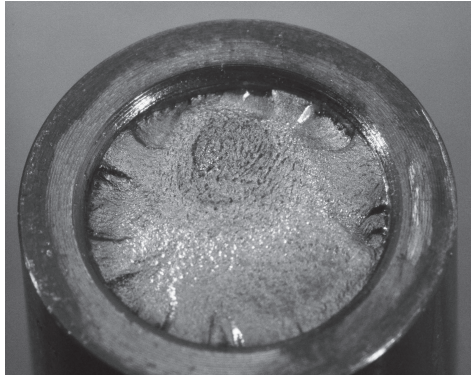
Figure 4.14: Fracture surface of specimen S19H6, \sigma_{y-RS} = 358MPa , n = 120, 376cycles , view of the hub side.
