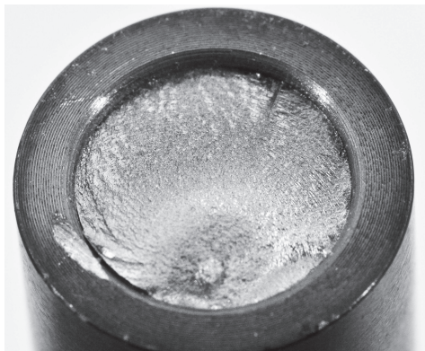
Figure 4.16: Fracture surface of specimen S28H2, \sigma_{y\_RS} = 211MPa , n = 1,518,646cycles , view of the hub side.
