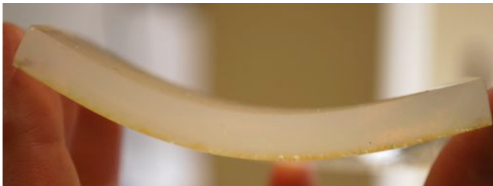
Figure 7.2. Hydrogel's capacity to perform uptake of hydrophilic materials, such as grime, is noticed (the film thickness is \approx 6 mm).
