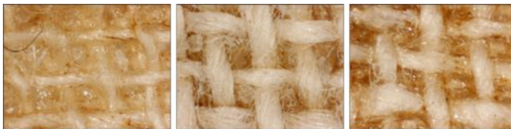
Figure 7.9. Optical microscopy images (x100 magnification) of the canvas with Plextol before (left) and after removal of the aged adhesive using EAPC system confined in H65 (center) and H50 (right) hydrogels.
