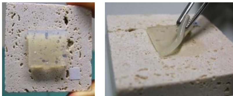
Fig. 1. Semi-IPN hydrogel (H65) on a travertine stone. On the left, the hydrogel applied in vertical position; on the right, the hydrogel removal is shown. It is worth noting that the stone surface is wet only in correspondence with the contact area.
