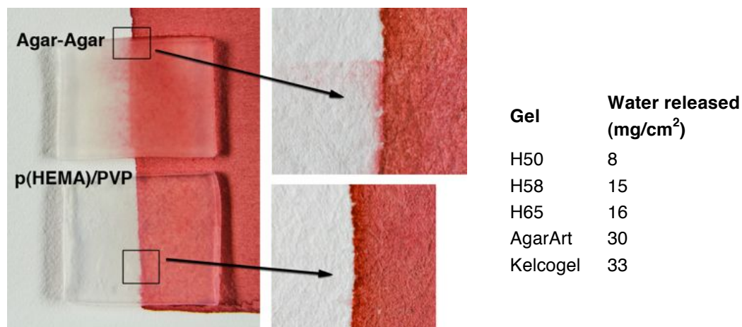
Figure 5.7. Five minutes application of agar-agar (2wt%) and H50 p(HEMA)/PVP hydrogel on paper painted with brazilwood ink, which is partially soluble in water. In the right, water release test results are presented for SIPN hydrogels and polysaccharide gels.
