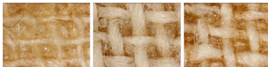
Fig. 5 Optical microscopy images ( \times 100 magnification) of the canvas with Plextol ® before ( left ) and after removal of the aged adhesive using EAPC microemulsion confined in H65 ( center ) and H50 ( right ) hydrogels
