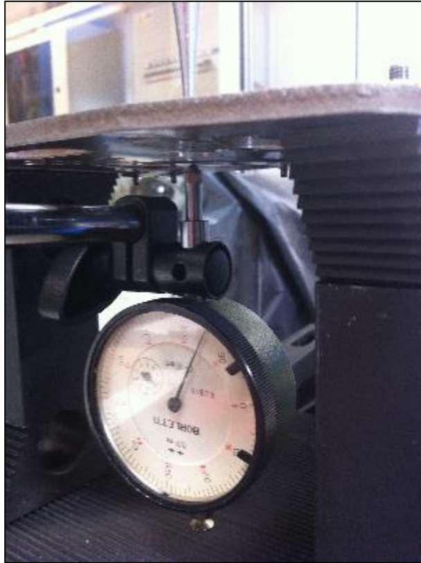
Figure 3.11 Detail view of the mechanical comparator tip positioning on the valve reed.
