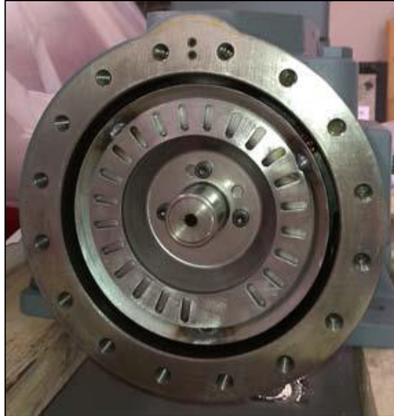
Figure 3.3 Circular ferromagnetic plate with 24-2 holes housed on the crankshaft.
