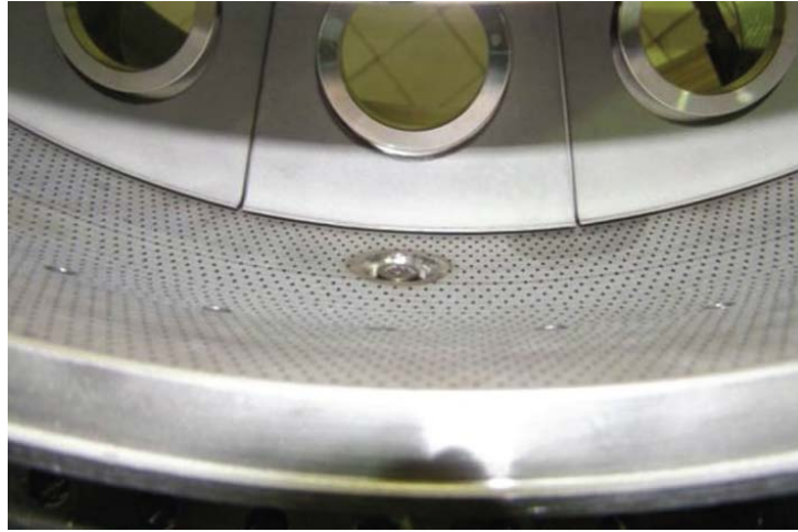
Figure 2.6: Combustor prototype of European Project NEWAC [57]
