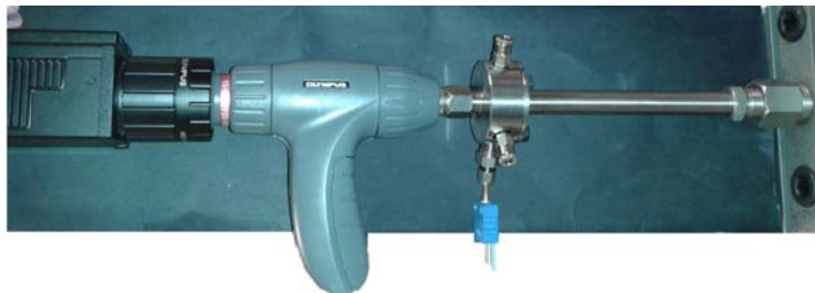
Figure 7.12: Camera boroscope provided with the cooling system and installed on Sector rig
