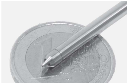
Figure 7.2: Typical 5-hole probe tip
