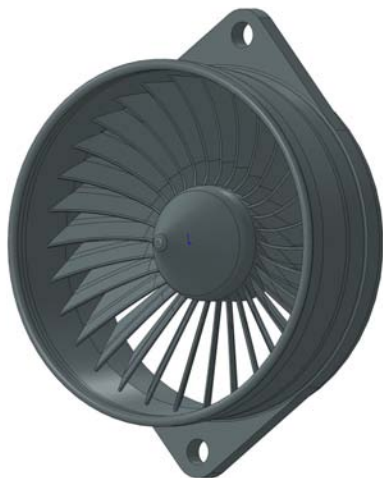
Figure 6.2: Sketch of a swirler of FACTOR combustor simulator
