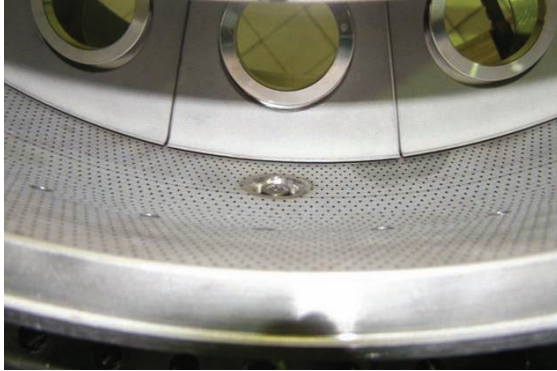
Figure 4.4: Liner cooling system of NEWAC combustor (courtesy of Avio Aero)
