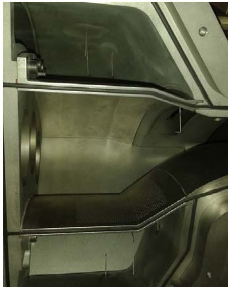
Figure 7.4: 5-hole probe installed in the outlet section of the CS
