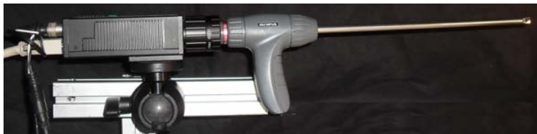
Figure 7.7: Rigid boroscope mounted on the PIV camera
