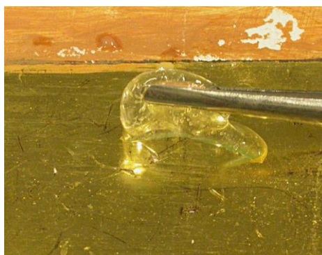
Figure 7.1.1. Exemplifying image showing the transparency of the HVPD systems (Carretti et al., J. Cult. Heritage , 2010, 11, 373).
