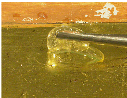
Fig. 1. Removal of a PVA/borax/water-based dispersion after it was in contact with a gilded surface for the minimum time necessary to soften the outermost surface layer. The gel was peeled easily from the surface by forceps.
