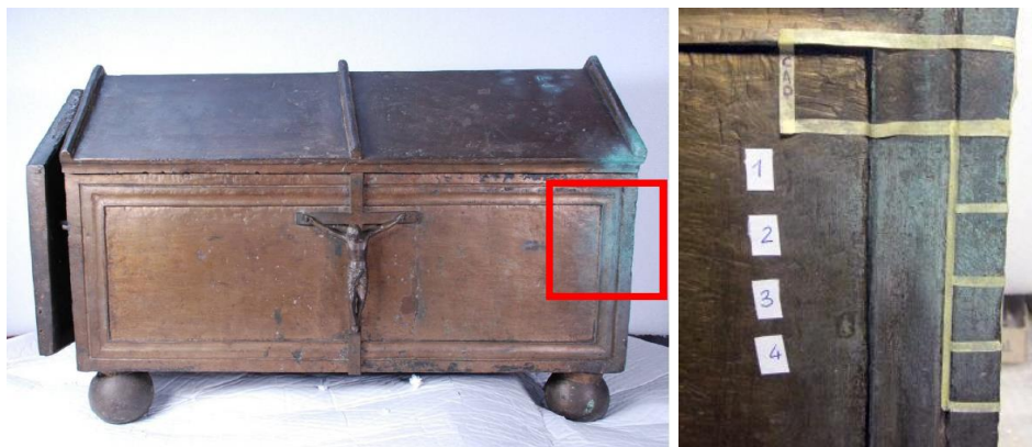
Figure 8.2.1. Left: “Cassetta-reliquiario con stemma dell’Arte di Calimala”; the area affected by bronze disease is highlighted by the red box. Right: magnification of the zone where the 4 cleaning tests were carried out.
