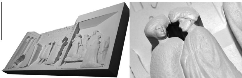
Fig. 18. Prototype of “The Healing of the Cripple and the Raising of Tabitha” obtained by using a CNC.
