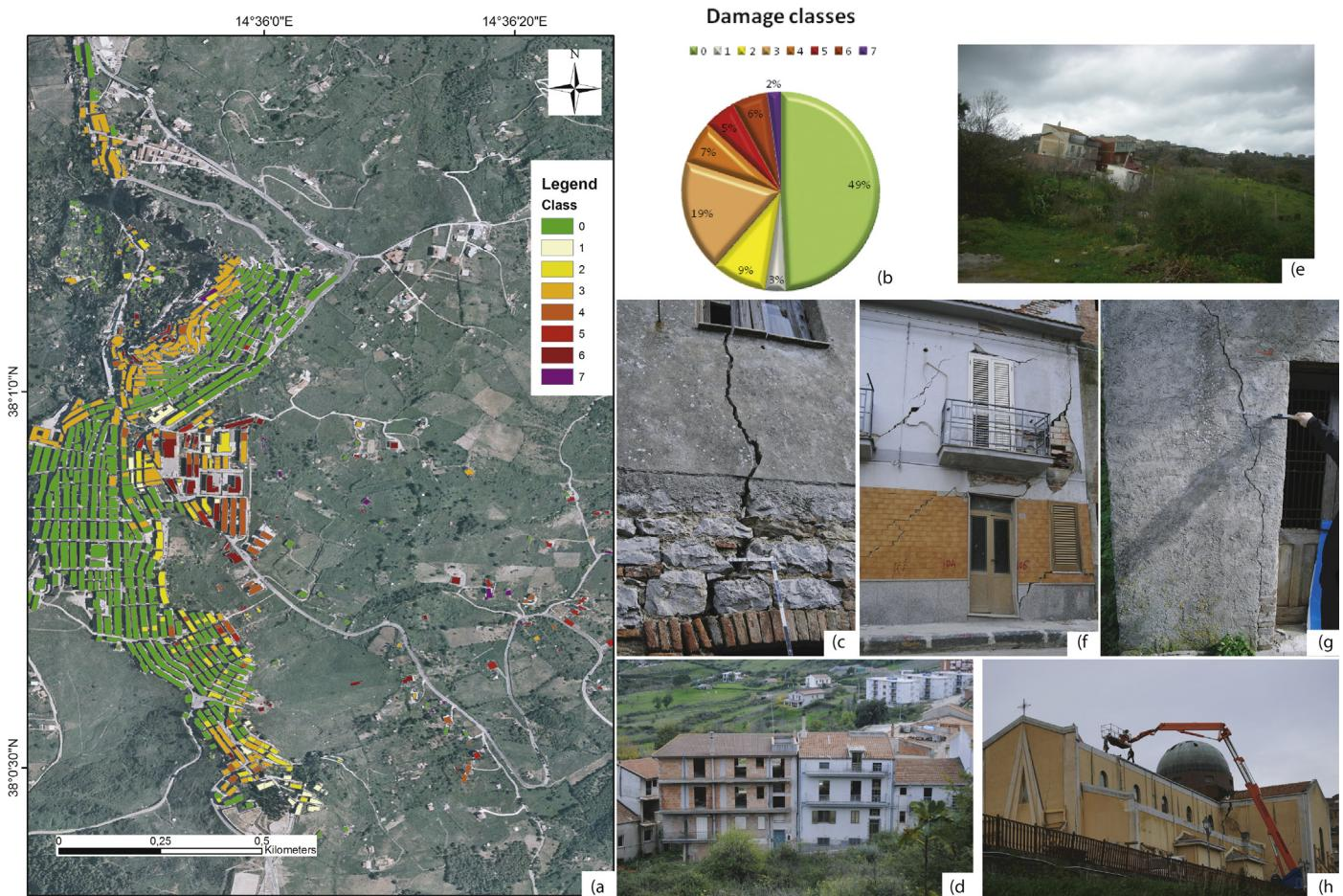
**Fig. 3.** Damage assessment map of San Fratello according to the degree of damages of Table 1 (a); and the related frequency of buildings considering the degree of damages (b). Some examples of the damages of San Fratello (c) class 3; (d) class 6; (e) class 7; (f) class 5; (g) class 2; (h) class 5.
