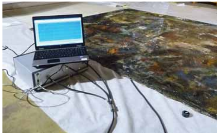
Fig. 7.9 - FORS instrumentation during the diagnostic survey of the Caverna dell'Antimateria
