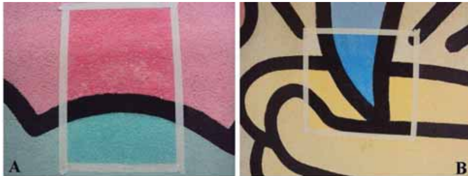
Fig. 6.18 - Cleaning tests carried out by means of a rigid rubber in the green/pink areas (A) and in the yellow/blue areas (B) (images acquired on 8 September 2011)
