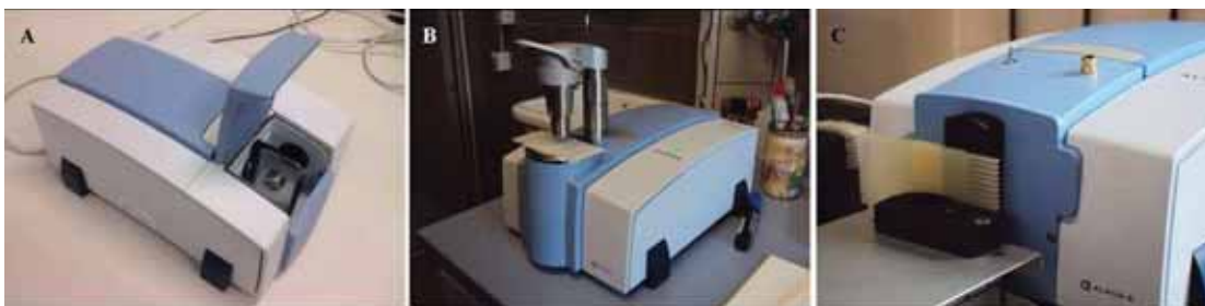
Fig. 3.5 - Alpha Bruker Optics spectrophotometer equipped with Trans (A), ATR (B) e TR (C) accessories
