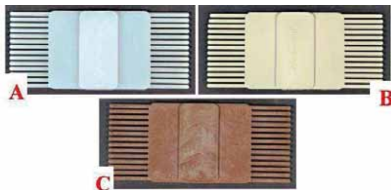
Fig. 3.4 - Resin Kit™, A) polystyrene medium impact; B) polyphenylene oxide; C) polyphenylene sulphide
