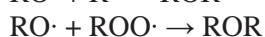
Fig. 2.5 - Radical reactions that take place during the autoxidation of an alkyd resin (van Gorkum and Bouwman, 2005; Soucek et al. , 2012)
