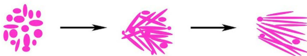
Figure 1.21 – Increase of NiMoO_4 nanorods length with the increase of US power
