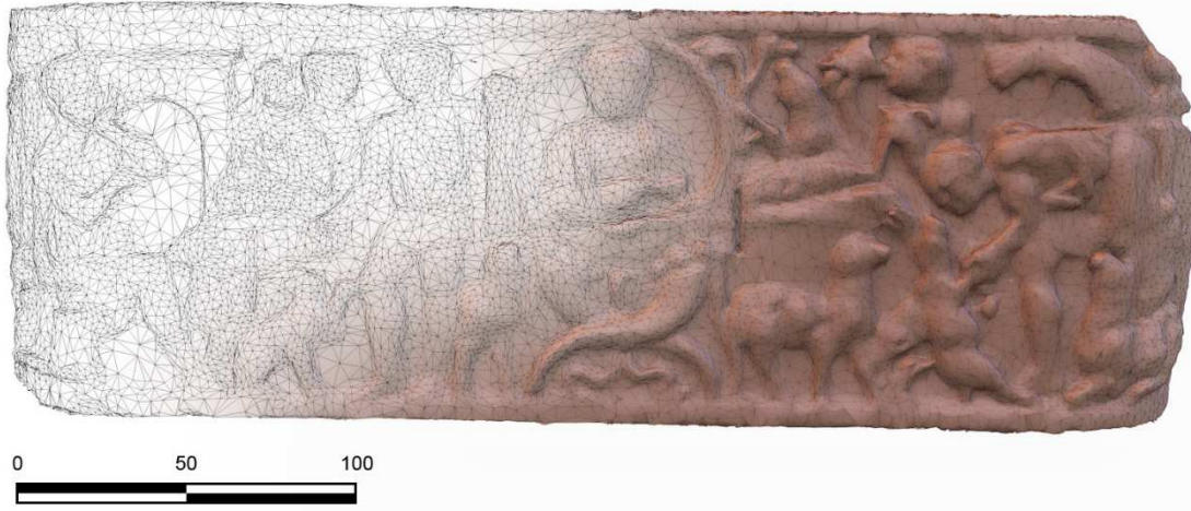
Fig. 12 – The decimated 3D model after the editing operations (reference scale in centimeters).
