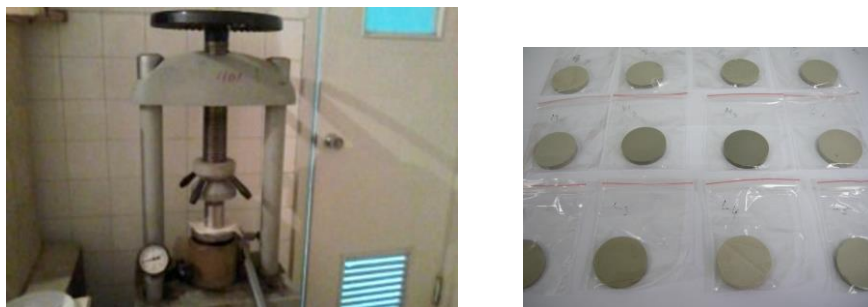
Photo 1. Pressing devices used for marine sediments. 2. Marine sediment pellets prepared until analysis in EDXRFS in the Center of Applied Physics, XRF latoratory,Tirana, Albania (For XRF and LIBS analysis)
