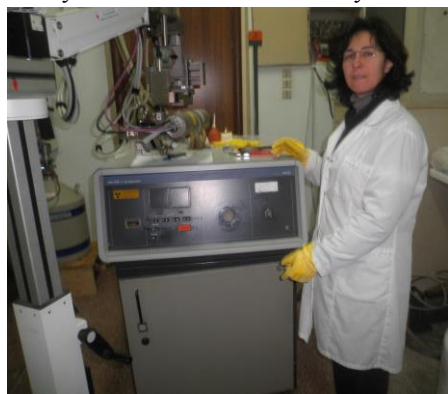
Photo. Philips 1729 - X-ray generator system in Tirana. Analyzing environmental samples by Energy Dispersive X-Ray Fluorescence
