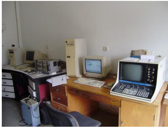
Photo. X ray fluorescence detection & elaboration system in the XRF laboratory, Center of Applied Physics, Tirana, Albania
