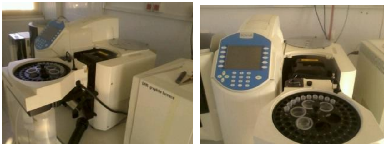
Photo THERMO SOLAR Graphite Furnace GF 95, Autosampler, AAS used Pb determination
