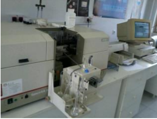
Foto AAS System of cold Vapor for analysis of mercury in marine sediment of Vlora. The device for the determination of mercury with cold vapor atomic absorption (photo I.Sino)
