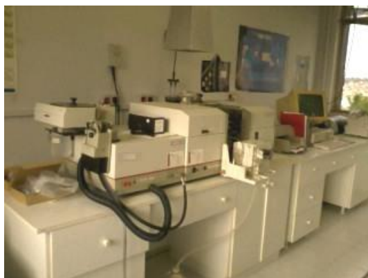
Varian Atomic Absorption Spectrometer AA200 / VGA 77 vapor Generation Accessory Determination of Hg concentration in Sea water . Mercury cold vapor technique. Analysing Hg in sea water in AAS/Cold vapor system (VGA-77)
