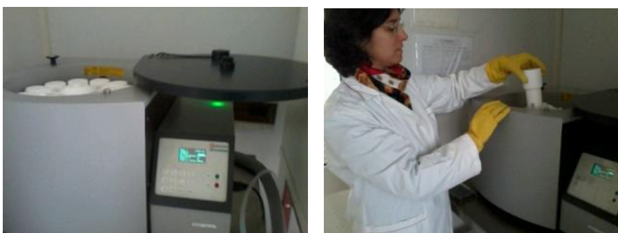
Foto. Digestion in Microwave oven BERGHOF, ISUV, (Toxicology & Quality department, Food Safety & Veterinary Institut, Tirana, Albania).
