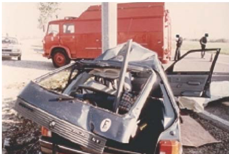
Figure 31: Collision with a lighting column: 2 fatalities [48]
