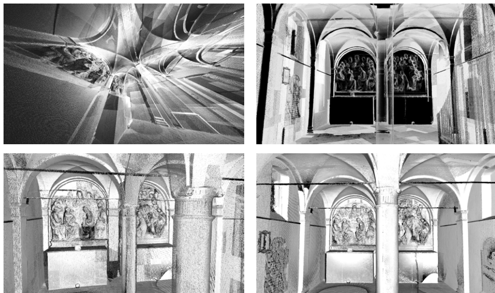
Fig. 1, 2, 3, 4 - Views from the first 3D laser scanner survey campaign, aligned pointclouds.
