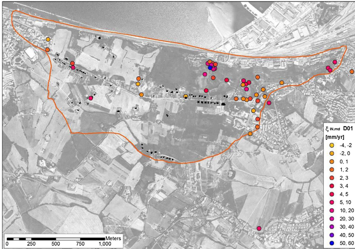
Fig. 6 Inclinometer-based estimates of \xi_{IN,md} at reference depth D01
