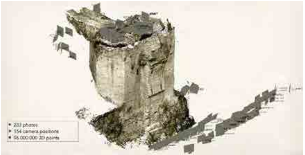
Fig. 11 – The process from the point cloud to the 3D model
