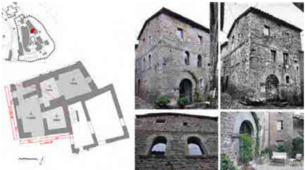
Fig. 9 – Dimensional analysis of the church of S. Matteo settlement, and maybe the Commune’s Palace. In the second part of the 14 th century Pietrabuona was definitively conquered by Florence. The fortress-gate system became a key feature of the final city wall. The architectural elements testify the Florentine presence and the circulation of new trends in cutting stone, construction and living. In the 16 th century Pietrabuona, like all the Valleriana valley, was finally a pacific area in the Florentine State and lost its military role.
