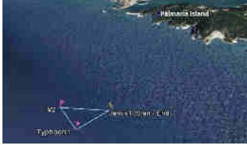
Figure 6.29: Layout of the autonomous mission: triangle-shaped path with vertices placed in the waypoints Janus1, M2 and Typhoon1
