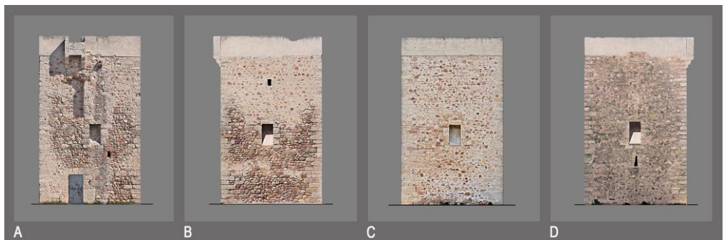
Fig. 1- Photogrammetric elevation of the Burriana Tower (Castellón) using a rectification system. A- West elevation. B- South elevation. C- East elevation. D- North elevation. (Graphic elaboration: R. Atzeni, V. Naldini, P. Rodríguez-Navarro).
