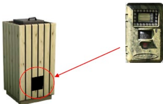
Fig. 1. Camera trap installing inside the waste basket
