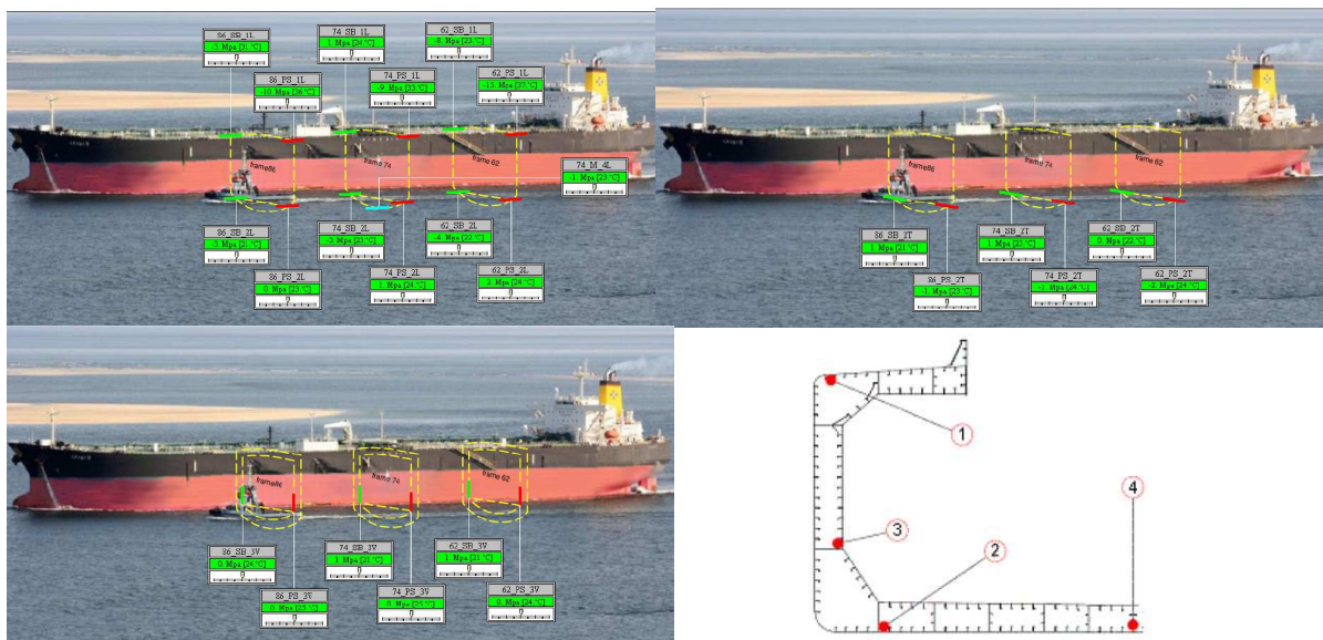
Figure 5. FSO Leonis and locations of strain gauges.
