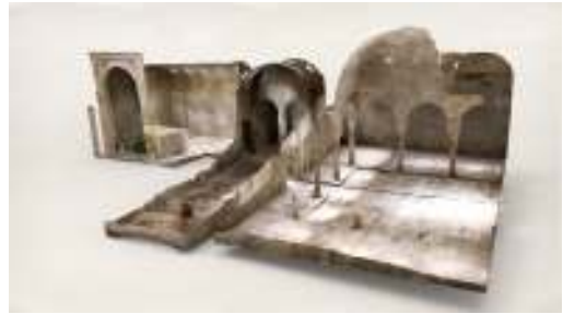
Figure 9 - Photogrammetry generated mesh with the texture coming from the shots automatically applied.
