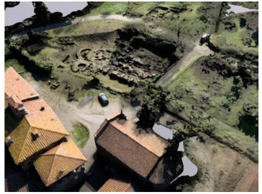
Figure 11 – 3D model created from the aerial (UAV) photogrammetry.
