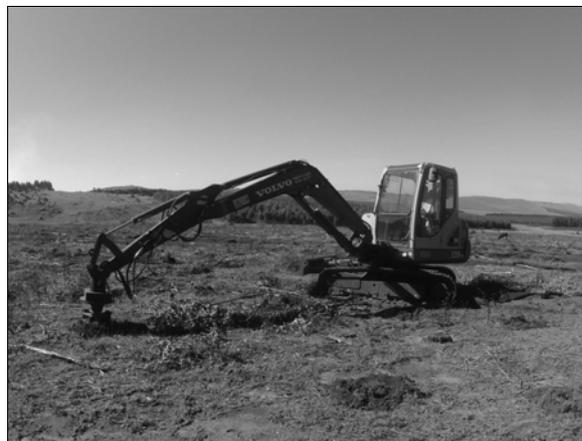
Figure 4. Modern mechanised pitting with mini excavator.
