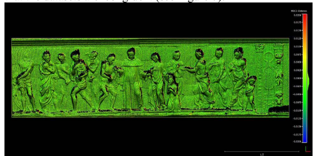
Figure 7. Comparison (based on signed distances) between scan models obtained with the C10 and 5010C
