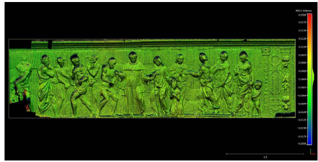
Figure 11. The outcome of the auto-calibration project demonstrates a very good conformity with the scan data assumed as the reference – Step 4
