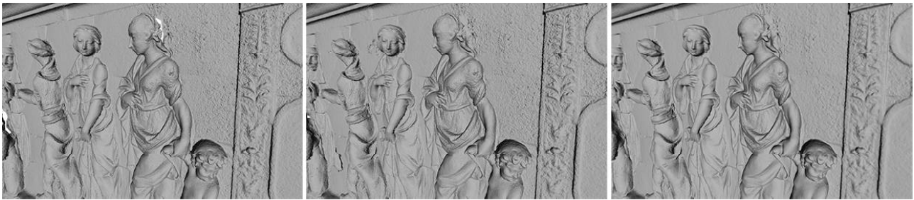
Figure 5. Comparison between meshing systems: (from left to right) model made using Photoscan, Meshlab (decimated after meshing), and Meshlab (decimated before meshing)
