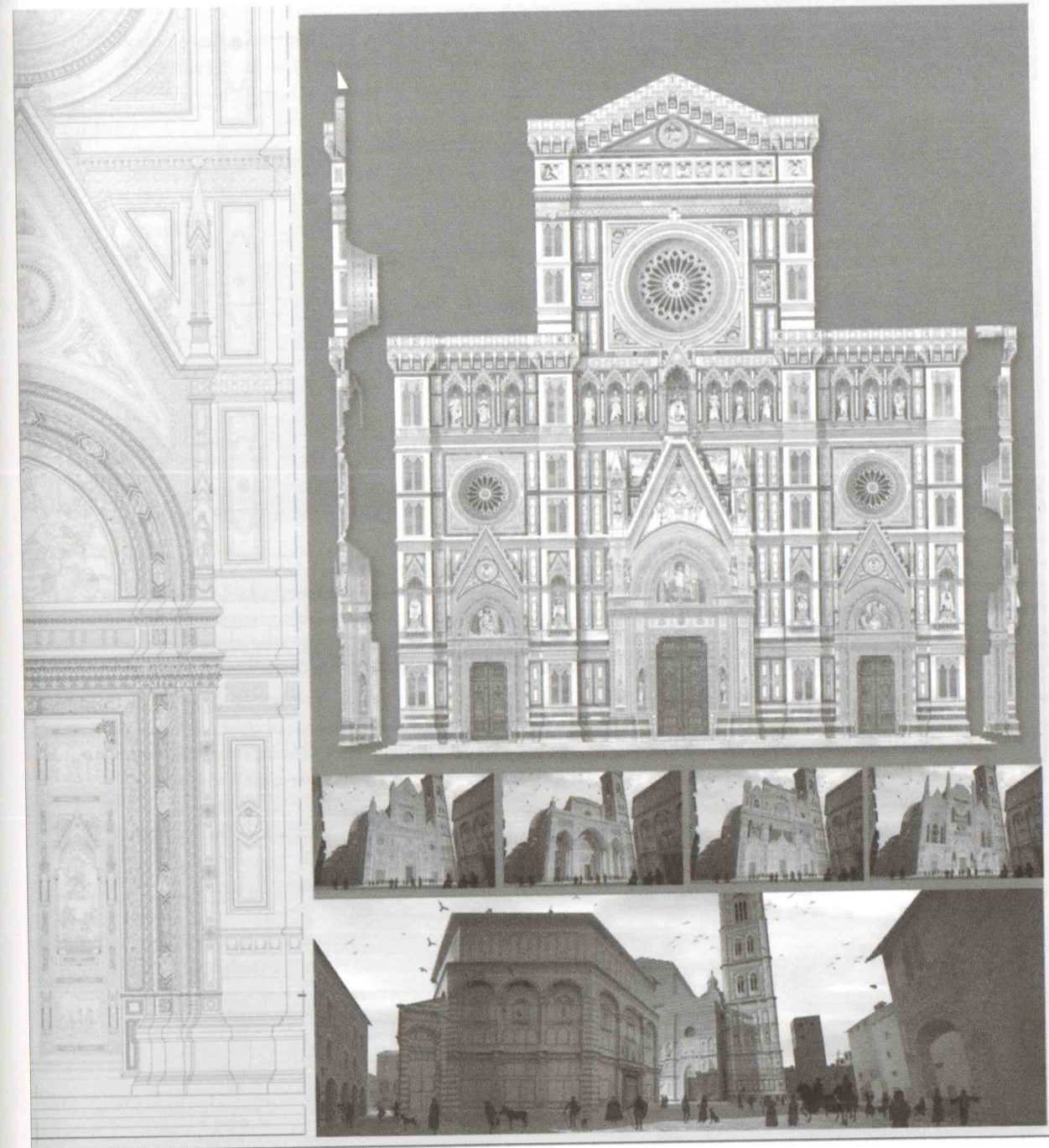
Fig. 1 The survey project for the documentation of the external facades of Santa Maria del Fiore Cathedral in collaboration with the Opera del Duomo in Florence. It allowed the digitization of the entire surface of the exterior stones. Through digital survey systems and digital photogrammetric work, it has possible to store the documented material through G.I.S. systems and to propose, through 3D modelling, a vast interactive scene.
