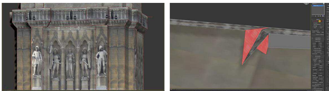
Fig. 5 – Above left: Compositing errors. Above right: self-crossing mesh.
