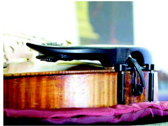
Figure 1: The dedicated designed and sensors equipped chinrest.
