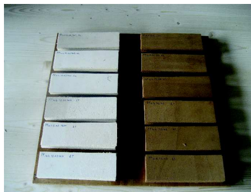
Figure 1: Heat treated (on the left) and untreated samples (on the right).
