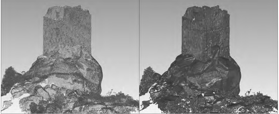
Fig. 3- San Giovanni Tower: the pointcloud and the mesh (Mancuso, Pasquali, 2016).
