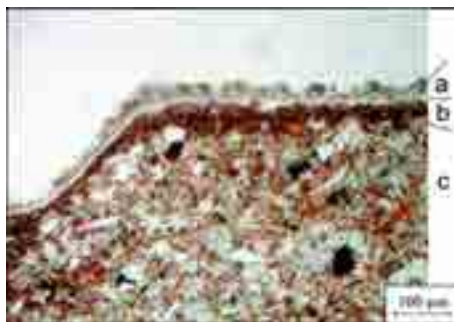
Fig. 9- Microstratigraphy (transmitted light, one nicol) of a microsample of a herringbone brick (Fig. 8): (a) degraded whewellite film; (b) film with ochres and weddellite; (c) brick.
