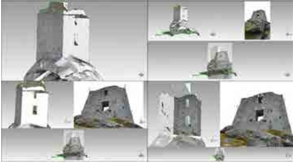
Fig. 4- The texture mapping process (Mancuso, Pasquali, 2016).
