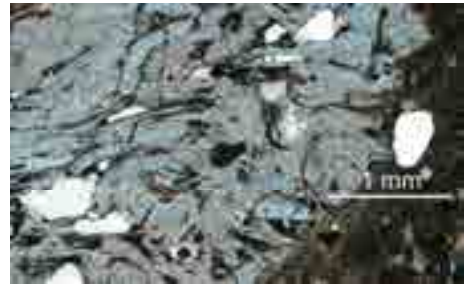
Fig. 8- Micro-photographs of volcanic aggregates from mortar of Nora theatre. Plain polars: fragment of obsidian glass with evident vacuolar and fluidal structure.
