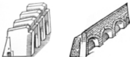
Fig. 3- Graphic description of the construction technique adopted in the strongholds of Sardinia (drawings by the treaty Della fortificazione delle città , published by G. Maggi in the 1564). Faced with masonry and filled with thick earth layers, it could absorb cannonballs.
