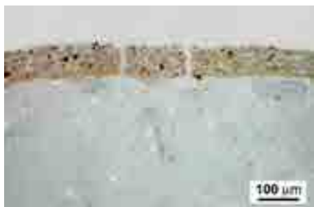
Fig. 7- Siena Cathedral main façade. Microstratigraphy (white-field reflected light) of the second type Ca oxalate film on marble. See text for explanations.
