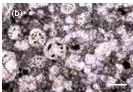
Fig. 7 a,b- Micro-photographs of mortar aggregates: (a) plain polars: vesicular black scoria immersed in the binder with reaction border; (b) plain polars: leucite crystals in the crystalline leucitite. Scale segment = 100 microns.
