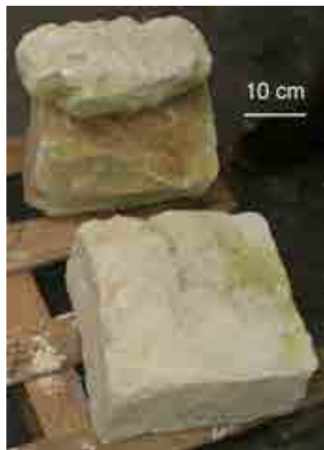
Fig. 2- Macro-photograph of original Pietra Cantone limestone ashlar taken from monument of tobacco factory during its restoration.
