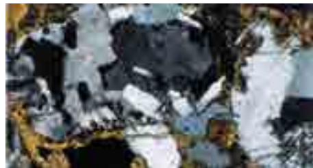
Fig. 6- Typical texture under the petrological microscope (crossed nicols) of the Montjuic Sandstone (“rebuig” variety), showing clast composition similar to the one in fig. 5, and pervasive presence of iron-rich cementation. During aggressive aqueous cleaning this component leads to the formation of permanent red stain fades in the rock, commonly arranged in a trend that mimics old sedimentary structures.
