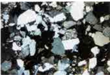
Fig. 5- Typical texture under the petrological microscope (crossed nicols) of the Montjuic Sandstone (“blancatge” variety), showing monocrystalline and polycrystalline grains of quartz, and minor presence of K-feldspar and plagioclase clasts, aggregated by silica cement. Note the scarcity of porosity.
