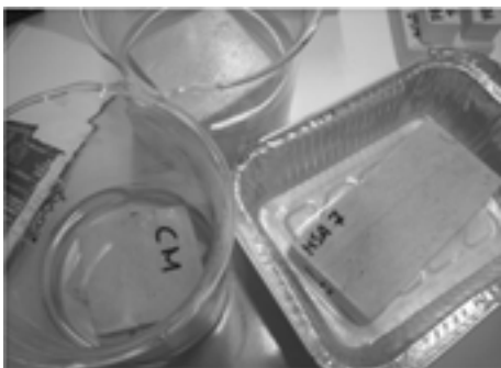
Fig. 3- Chemical treatment by immersion of cubic and prismatic limestone specimens.
