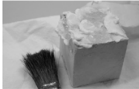
Fig. 4- Cubic limestone specimen with edge 5 cm treated with nano-gel.
