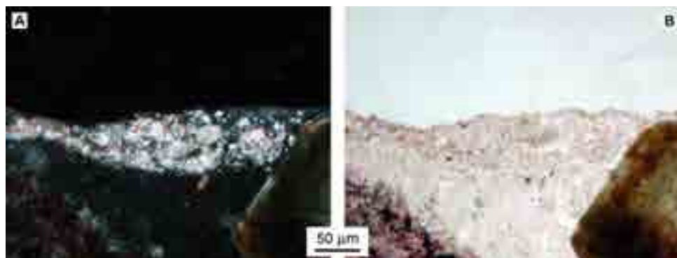
Fig. 12- Sant'Antioco di Bisarcio Basilica (north Sardinia). Sample A85: photographs on thin section of a type1 film under the polarized light microscope; single layer is observed on the rock surface. A) Transmitted light, converging lens, crossed nicols – B) Transmitted light, one polarizer, converging lens.
