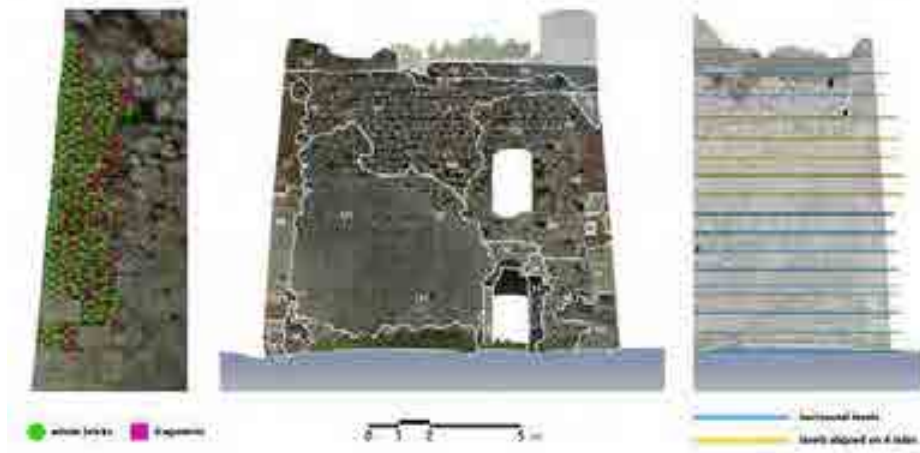
Fig. 6- Stratigraphic and typological analysis of the elevations.
