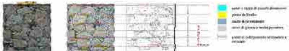
Fig. 11- Masonry frame and analysis of the function of the constituent elements.
